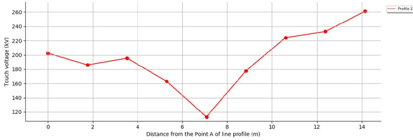
Figure 14 – Maximum touch voltage during the response along the line profile
