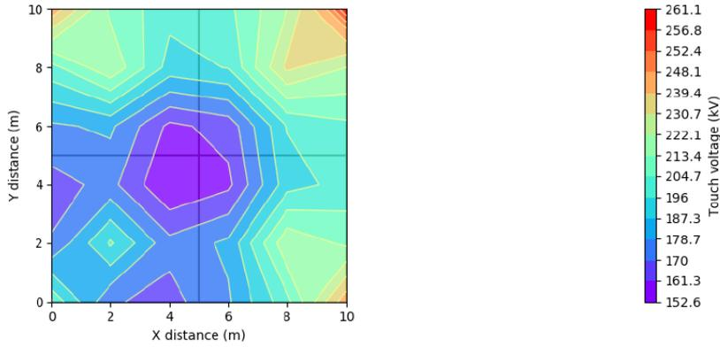
Figure 13 – Maximum touch voltage (kV) during the response of the rectangle profile
