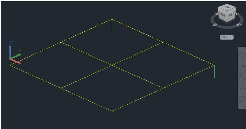
Figure 1 – Example earthing system drawn in CAD
