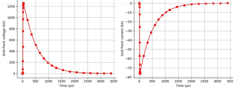
Figure 15 – Grid point response at faulted segment
