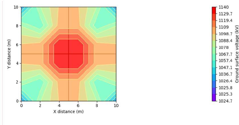
Figure 11 – Maximum surface voltage (kV) during the response of the rectangle profile
