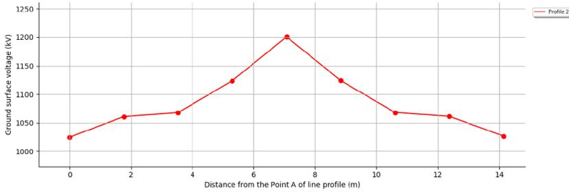
Figure 12 – Maximum surface voltage during the response along the line profile
