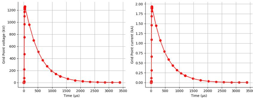
Figure 16 – Grid point response away from faulted segment
