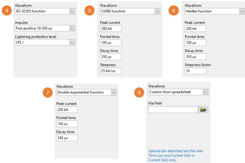
Figure 3 – Input waveform types
